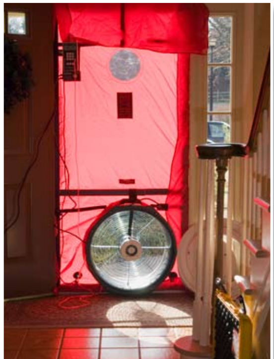
A blower door test like this one can detect air leaks in your home.
