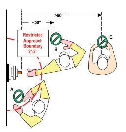
**A)** The work is inside the Restricted Approach Boundary (RAB). Class 2's and sleeves, tested overshoes, and a trained watch person are required. Exposed parts must be covered or barricaded. NO intentional contact with live parts is allowed.
