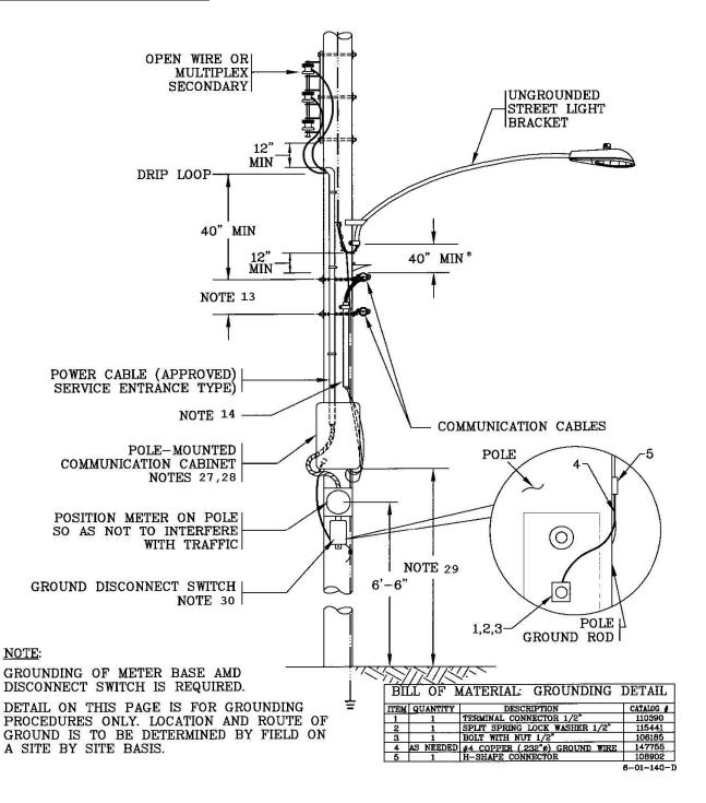
\*Note: 40" minimum may be reduced to 4" if the streetlight bracket is grounded. A minimum clearance of 12" is still required from the communication cable bracket to the streetlight drip loop. To effectively ground street light bracket, use PPL CID 1029820.
