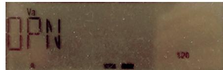
The next screen will say "CLS" if the switch inside the meter is **closed** and power is flowing to the property. **It will say "OPN"** if the switch is **open** and no power is being delivered. If your account is in good standing, you should always see "CLS."
