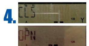
The next screen will say "CLS" if the switch inside the meter is closed and power is flowing to the property. It will say "OPN" if the switch is open and no power is being delivered. If your account is in good standing, you should always see "CLS."
