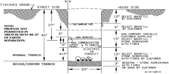
\* MAINTAIN 12" TOTAL SEPARATION FROM TOP OF CONDUIT TO CLOSEST UTILITIES. IF JOINT UTILITY IS LOCATED DIRECTLY ABOVE, WITH NO HORIZONTAL COMPONENT TO SEPARATION, TRENCH DEPTH MAY NEED TO BE INCREASED.
