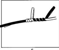
5. Using the other end, repeat the process outlined in step 2. After concluding this process, both ends should be sticking up as shown.
