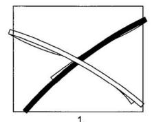
Take each end of the flat pulling line to be spliced, and without twisting, fold so that each end is doubled for approximately 18 inches. Take the end on the right and cross it over the end on the left.
