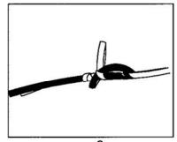
6. Insert the tape end used in step 5 down through the same hole where the looped lines crossed initially, as in step 3.
