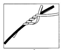
3. Without twisting, bend the wrapped end back and insert it between the looped lines at the point where they crossed initially (in step 1).
