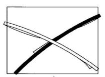
Take each end of the flat pulling line to be spliced, and without twisting, fold so that each end is doubled for approximately 18 inches. Take the end on the right and cross it over the end on the left.
