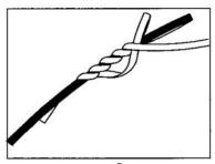
Without twisting, bend the wrapped end back and insert it between the looped lines at the point where they crossed initially (in step 1).
