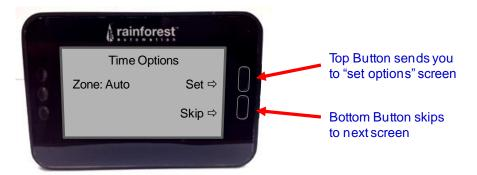
e. If you need to change the time zone, press the Top Button and follow the directions for the *Set Time Options* screen in the **Configurations Screens** section of this manual. Otherwise, press the Bottom button to see the *Power Source* screen:
