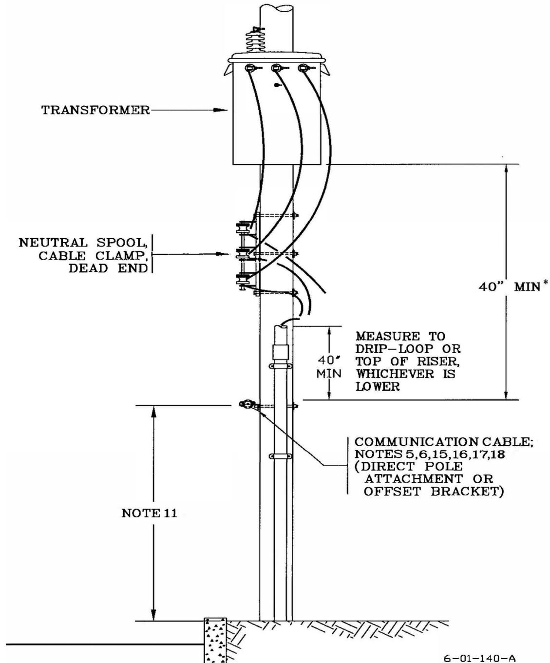
\*Note: Can be reduced to 30" minimum to neutral, primary underground cable or primary cable assembly if attaching cable company bonds to PPL EU's vertical ground wires. See Note 31.
