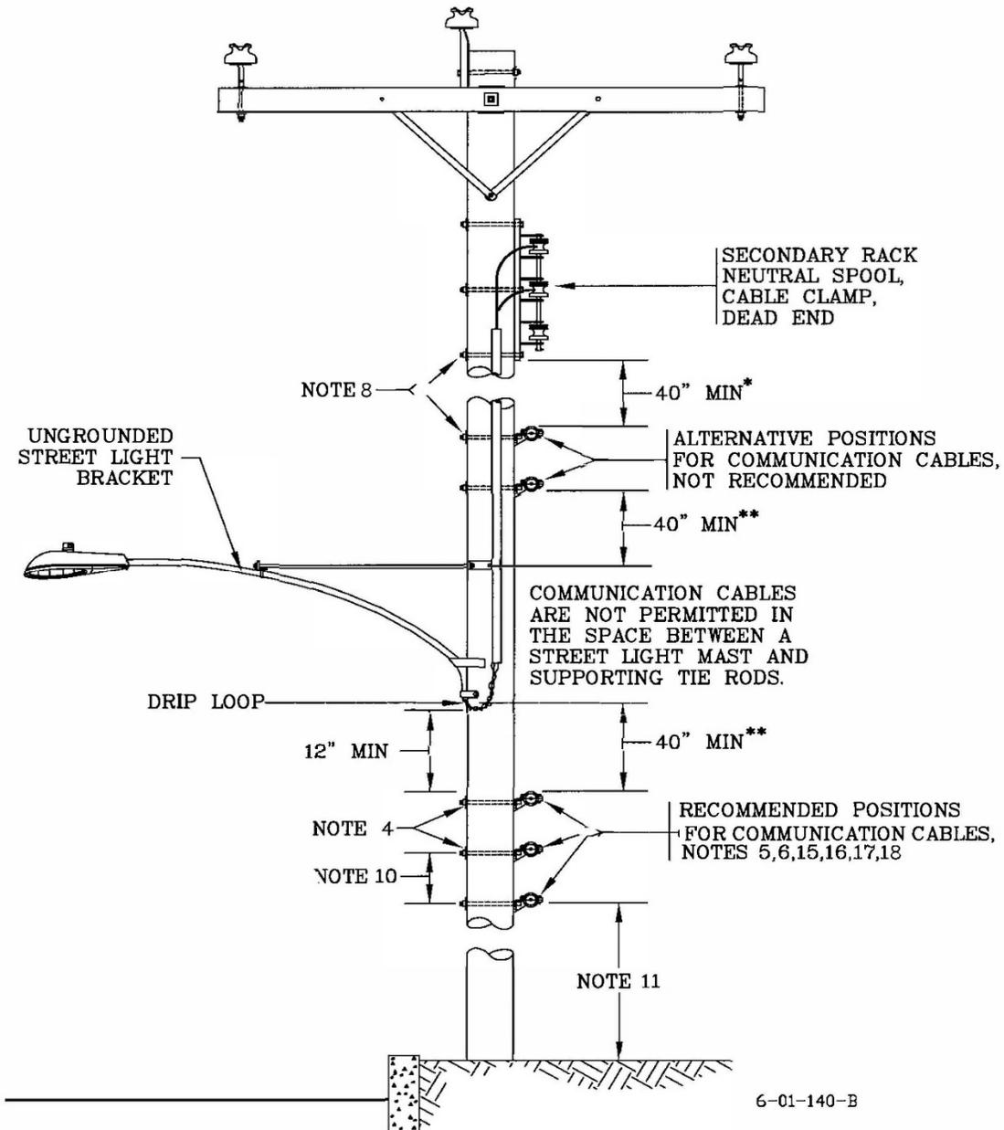
\*Note: Can be reduced to 30" minimum to neutral, primary underground cable or primary cable assembly if attaching cable company bonds to PPL EU's vertical ground wires. See Note 31.
