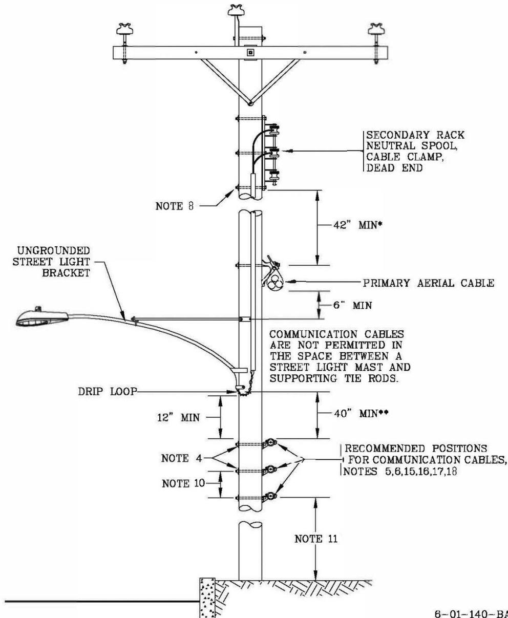
\*Note: Can be reduced to 30" for spans under 175 feet.
